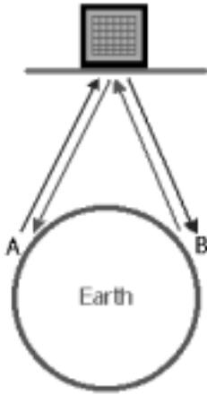
**Figure 3. Radio "repeater" functionality of DARTSAT.**
